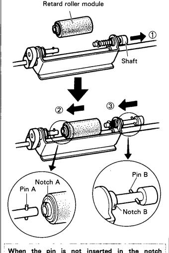
When the pin is not inserted in the notch properly, it may cause double feeding or a paper jam.
