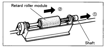
12 Take out the retard roller module in the optional "Roller Exchange Kit (KV-SS044)".
