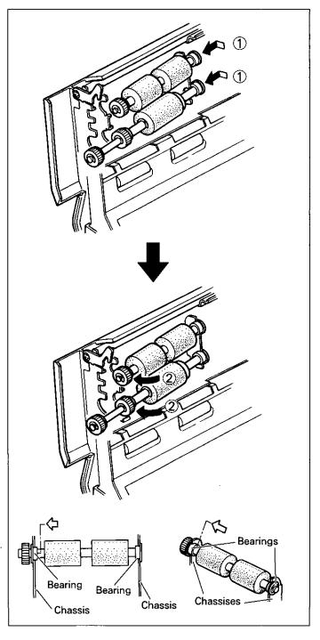
8 Tilt the paper feed conveyor at a slight angle pointing downward and attach it as shown in the diagram to the right.
