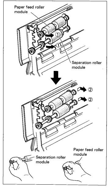
Open the optional "Roller Exchange Kit (KV-SS044)", and take out the paper feed roller module and separation roller module. For supplies and accessories: Call 1-800-346-4768 (U. S. A. only) or your dealer.
